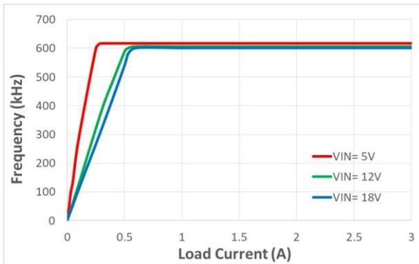
**Figure 3. Frequency vs. Load Current**
