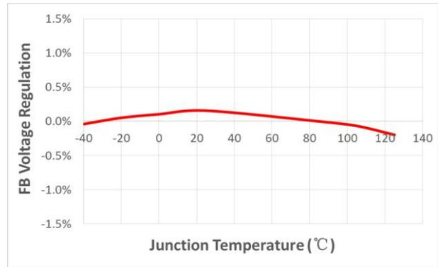
**Figure 2. FB Voltage Regulation vs. Junction Temperature**
