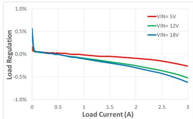
**Figure 4. Load Regulation vs. Load Current**
